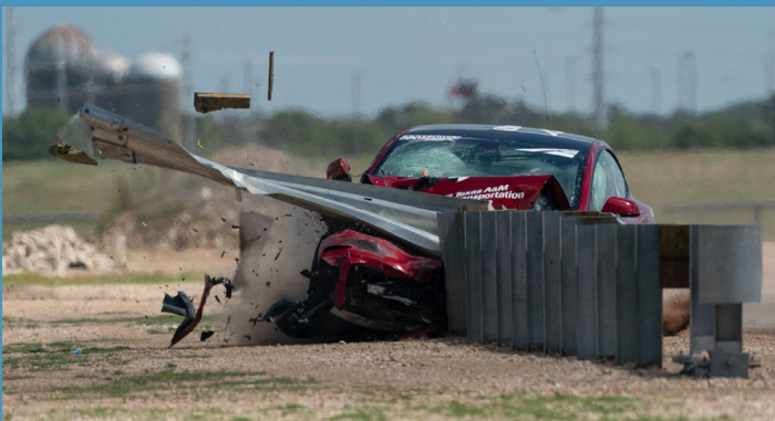
TTI researchers subjected a Tesla Model 3 to a 62-mph impact at a 25-degree angle with a thrie beam guardrail system – the same conditions used for MASH crash testing. The impact ruptured the thrie beam rail and allowed the test vehicle to penetrate through the barrier.
